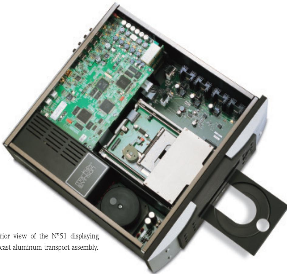
Interior view of the N°51 displaying the cast aluminum transport assembly.
