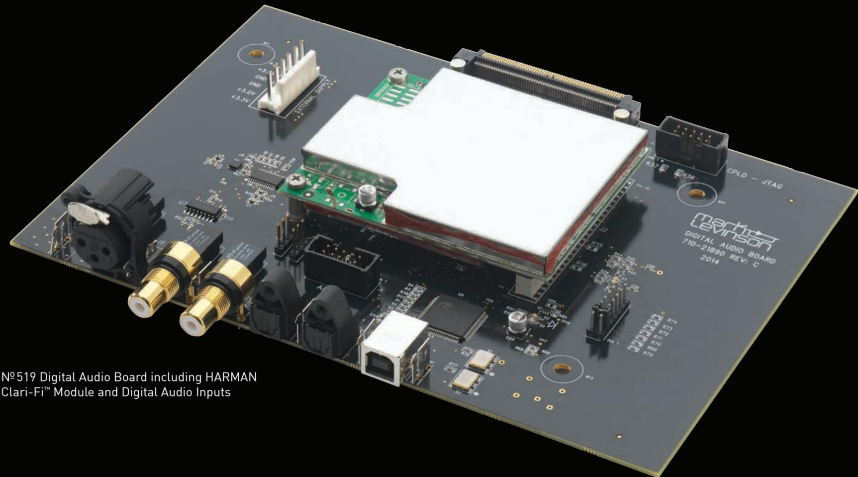
N°519 Digital Audio Board including HARMAN Clari-Fi™ Module and Digital Audio Inputs
