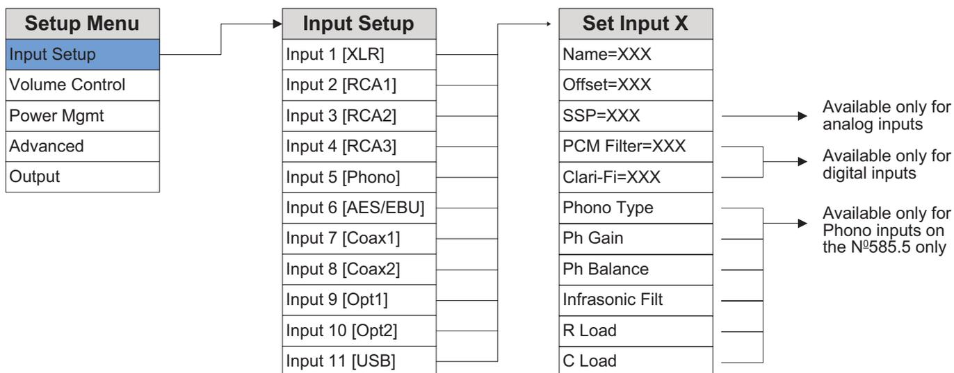
The Input Setup menu allows you to customize the following parameters for the selected input:
