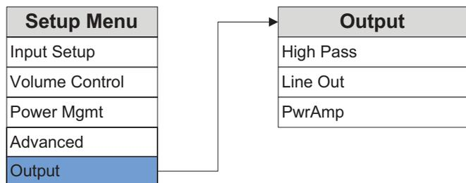
The Output section of the Setup menu lets you configure the N°585's outputs.
