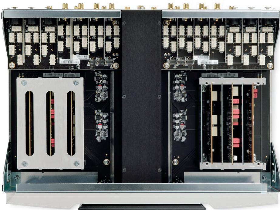
**RIGHT:** Local relay switching in the preamp proper connects to and from line and MM/MC phono amplifier cards (right channel enclosure opened for clarity in this picture)
